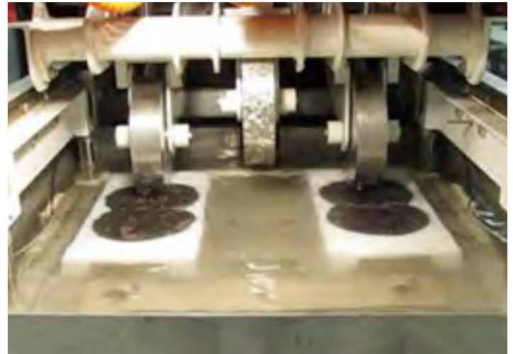
Figure 1. Hamburg Rutting and Stripping Test Performed on Asphalt Mixture
