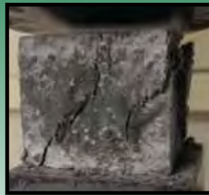
Figure 2a. Poly (vinyl alcohol co-ethylene) based concrete specimen
