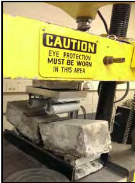
Figure 1. Flexure test of PMC beam
