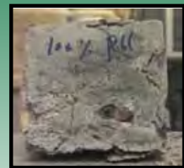
Figure 2b. Polyurethane based concrete specimen
